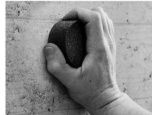
Fig. 5.1 Preparing the test surface
