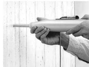
Fig. 5.2 Deploying the impact plunger (1)
