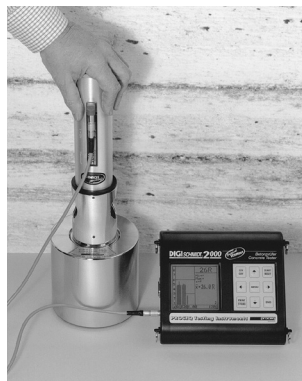
Fig. 6.1 Performance check of the concrete test hammer
